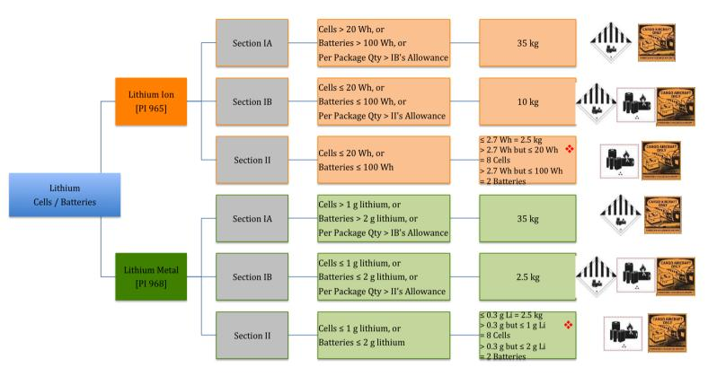
Cells and batteries within the three ranges of watt-hour rating or lithium content listed must not be combined in the same package (i.e. shippers must not combine 4 cells with no more than 20 Wh together with 1 battery with no more than 100 Wh in a single package).
