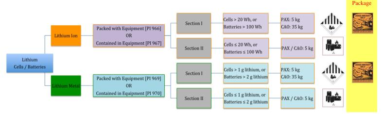
**NOTE**: **"Equipment**" means the device or apparatus for which the lithium cells or batteries will provide electric power for its operation.
